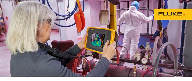
Ultrasonic tools use microphones to identify the sounds associated with escaping air/gas in a range of about 38 to 42 kHz. They convert sound captured in this range into audible sound and therefore rely on human hearing to identify whether a noise is a leak or not. That makes the detection subjective, and reliant on enhanced skills and training.
